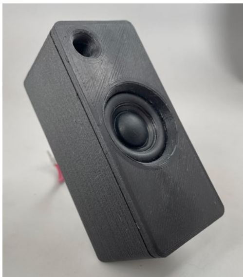
Satellite speaker enclosed with a black ABS plastic enclosure
